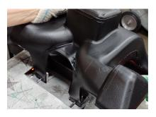
In this example a blow molded part that was automatically lanced is being checked for the proper position of two holes that are critical for final assembly. If the part is cooled too slowly or quickly after molding the hole locations change, causing defects. This type of phenomenon occurs in all molding processes, MIG and TIG welding, and castings.
