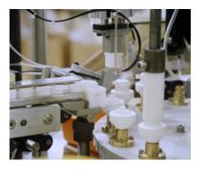
For this assembly operation part dimensional variations or flash will result in mis-feeding, mis-placement, or failure to complete cycle. All will cripple the assembly output. This is true of any assembly process including welding.
